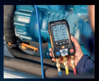
Thanks to Bluetooth® 5.0, the new digital manifolds with an extra-large display and rugged safety housing are also suitable for wireless measurement. You save valuable time and avoid stress in the installation, maintenance, and servicing of refrigeration systems and heat pumps. All important measurement programs are already stored in the manifold, as well as the right refrigerants for different systems.
