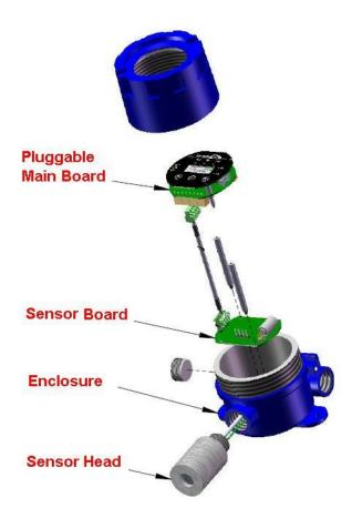
Important: Transmitter must be calibrated when the sensor is replaced.
