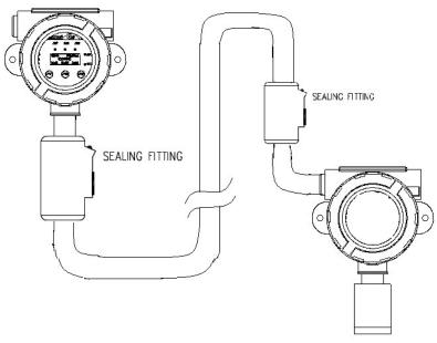
The Smart Sensor Head can be equipped with B8 locally or remotely. For installations where the smart sensor head assembly will be mounted remotely from B8, the max distance between B8 and Remote Smart Sensor Head is 100 meters. The Remote Smart Sensor Head Assembly is not included in the B8 standard package, it must be ordered separately.
