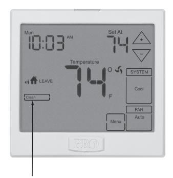
Hold down **CLEAN** for 3 seconds, to reset filter reminder.
