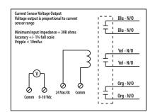
**Coil Current:** 210 mA @ 24 Vac 154 mA @ 30 Vdc Coil Voltage Input: 24 Vac/dc ; 50-60 Hz Drop Out = 3 Vac / 3.8 Vdc Pull In = 20 Vac / 20 Vdc
