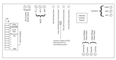
NETWORK COMPATIBLE RELAY / CURRENT SENSOR COMBOS
