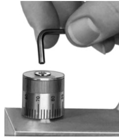
Figure-14 Dial Adjustment of Three Stage Thermostats.
