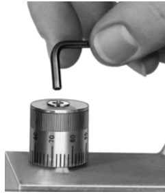
Figure-11 Dial Adjustment of Two Stage Thermostats.
