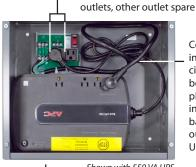
Cord from interface circuit board plugged into battery backed up outlet of UPS.
