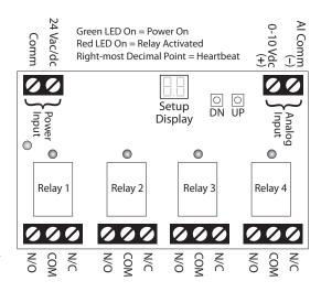
FOR SUPPLY CONNECTIONS USE #14 AWG OR LARGER WIRES RATED AT LEAST 75°C (167°F).
