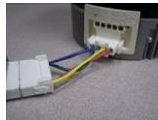
figure 3 installed harness assembly
