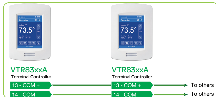
Figure-7 MS/TP Connections
